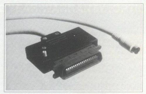
Revised model with configurable dial and all-in-one 9 & 24-pin support
